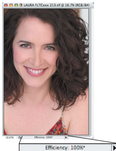
FIGURE 6.1 If Photoshop's Efficiency meter drops below 100 percent, you know that it can no longer keep all of its image data in RAM. Less than 100 percent efficiency means it must spool information to disk, which leads to slower performance. Keeping an eye on the Efficiency gauge is a good way to determine if your system could use more RAM.
